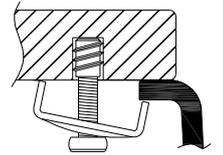
You should confirm with your client if the worksurface cutout is to be cut flush, inside or outside this suggested perimeter shape & size.
