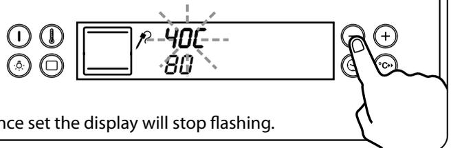
**Step 7.** Press the "Temperature" button again. The probe temperature will show.
