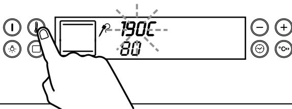
**Step 5.** Press the "+" button to increase the temperature.
