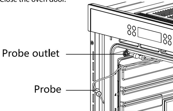
**Step 2.** If fitted correctly, the probe symbol will show on the display.
