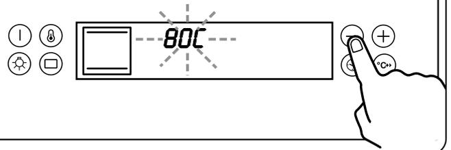
**Step 7.** Firmly press the rapid heat button until a tone is emitted.
