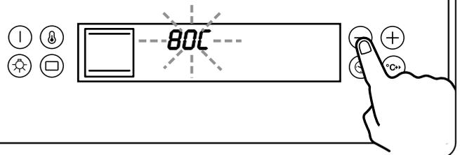
**Step 8.** Press the temperature button to start and confirm selection.
