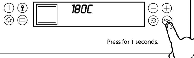
**Step 7.** Alarm will sound when the oven has reached the desired temperature.
