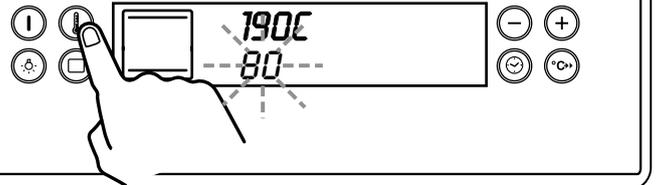
**Step 8.** Alarm will sound when the internal temperature of the probe has been reached.
