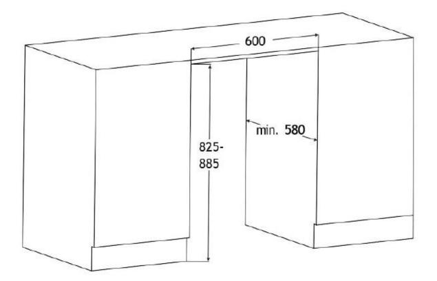
PLEASE NOTE - DIMENSIONS CAN VARY BY +/- 2mm DUE TO MANUFACTURING TOLERANCES, ALL DIMENSIONS ARE GIVEN IN MILLIMETRES (mm)
