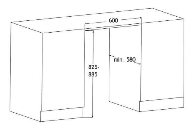
PLEASE NOTE - DIMENSIONS CAN VARY BY +/- 2mm DUE TO MANUFACTURING TOLERANCES, ALL DIMENSIONS ARE GIVEN IN MILLIMETRES (mm)
