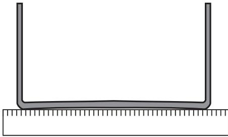
The very best pans have bases that are very slightly curved up when cold (**Fig. 2.3**). If you hold a ruler across the bottom you will see a small gap in the middle. When they heat up the metal expands and lies flat on the cooking surface.
